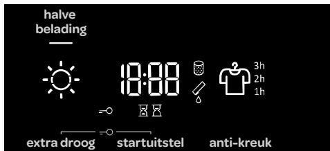
When the set delay time expires, the selected drying programme will start automatically.
