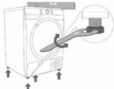
1. Rotate the adjustable feet with a spanner.
