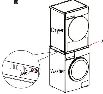
If the dryer base is metal, only tighten the front two screws A.
