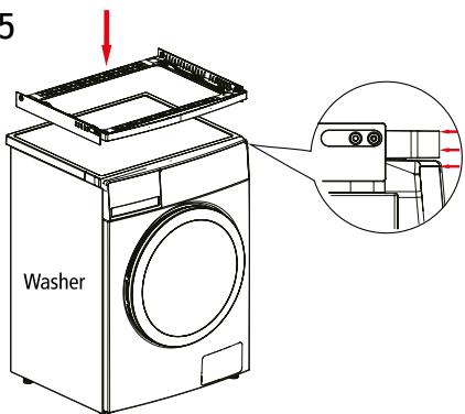
Note: Align the bracket B and the washing machine before sticking the bracket B with the stickers on the bottom of the bracket
